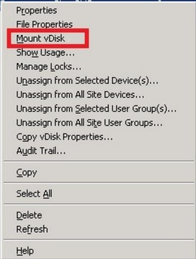
A context menu is displayed over the VMNX row of the table. The menu items are: Properties, File Properties, Mount vDisk (highlighted with a red box), Show Usage..., Manage Locks..., Unassign from Selected Device(s)..., Unassign from All Site Devices..., Unassign from Selected User Group(s)..., Unassign from All Site User Groups..., Copy vDisk Properties..., Audit Trail..., Copy, Select All, Delete, Refresh, and Help.
